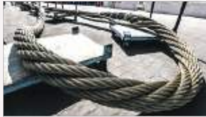
LIFT CABLE LAID GROMMETS & SLINGS
